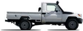
Land Cruiser 79 Pick-Up Single Cabin/Cabine Simple/Cabina Simple 4.2 litre Diesel 3 seater/places/plazas / 4x4 ●● Code/Código: HZJ79L/R-TJMRS
