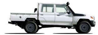
Land Cruiser 79 Pick-Up Double Cabin/Double Cabine/Doble Cabina / 4.2 Diesel 6 seater/places/plazas / 4x4 ●● Code/Código: HZJ79L/R-DKMRS
