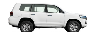
Land Cruiser 200 Station Wagon STD V8 / 4.5 Twin Turbo Diesel Manual/Manuelle/Manual 5 seater/places/plazas / 4x4 ●● Code/Código: VDJ200L-GCMNZV
